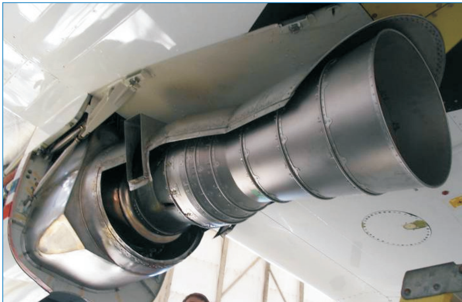
CN-235 Centre Body Tailpipe IRS (engine cowling removed)
